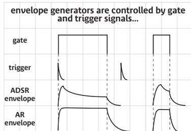
A device whose output is intended to control some time-varying attribute of an event is called an *envelope generator*. These are sometimes referred to as *transient generators*, to call attention to the fact that their output is not constant but transient.
