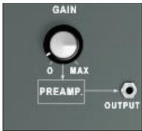
The *Preamp* section controls the gain of the audio signal(s) from the track in which the TimewARP 2600 is running. A rotary knob labeled *Gain* adjusts the signal level.
