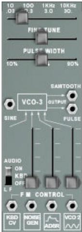
VCO 3 generates sawtooth, pulse, and sine outputs; the pulse width is manually variable. The sine output is a TimewARP 2600 extension; the original ARP 2600 VCO3 provided just sawtooth and pulse outputs.
