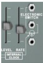
The *Internal Clock* is a manually controlled low-frequency square-wave oscillator. It is the default trigger source for the *S/H* device. It is also hardwired as the clock source for the *Electronic Switch*.
