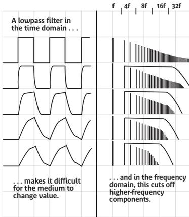
Any device or mechanism that passes along slower motions better than faster ones can act as a lowpass filter.
