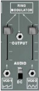
The *Ring Modulator* is essentially a multiplier; from its two inputs A and B it produces the output function  $A \times B / 5$ . The kind of transformation this effects on input signals depends to a large extent on what they are and on whether the modulator is AC or DC coupled to them. This is selected by the *Audio/DC* switch at the bottom of the modulator.
