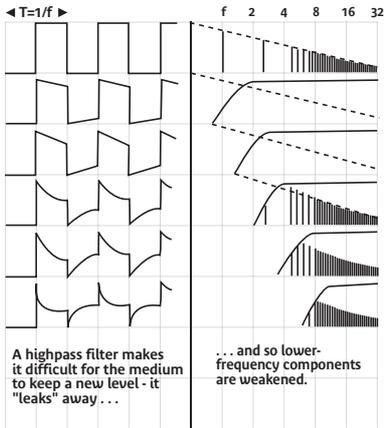
Any device or mechanism that passes along faster motions better than slower ones is a highpass filter.
