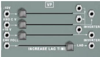
The *Voltage Processors* are simple utility functions for mixing, inverting, and shaping signals.
