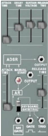
The *Envelope Generators* generate transient, positive-going waveforms, with controllable rise and fall times. They are used primarily with the *VCF* and *VCA*, in generating events whose time-varying spectrum and amplitude must be accurately and repeatably controlled. The output from each generator is a positive-going signal whose rise and fall time is set by slide controls on the generator, and whose onset and overall duration is determined by a gate signal.
