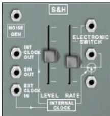
The *Sample & Hold Module* produces stepped output signal levels, by sampling the instantaneous value of any signal at its input. The stepped levels produced in this manner are useful for controlling oscillator and filter frequencies and – occasionally – *VCA* gain.
