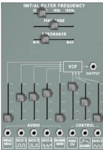
The *Voltage Controlled Filter* has variable cutoff frequency ( $F_c$ ) and resonance ( $Q$ ). The response below  $F_c$  is flat down to DC; above  $F_c$  the response falls off at 24Db per octave.  $F_c$  range is from 10Hz to 10KHz without control voltages; under voltage control,  $F_c$  can be driven as far down as 1 Hz and as high as 20KHz.
