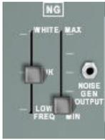
The *Noise Generator* has two manual controls: one for spectral balance (“color”) and one for output level.
