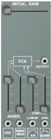
The *Voltage Controlled Amplifier* has a maximum gain of unity and a dynamic range of 100Db. With the initial gain control at maximum, and with no control input, the VCA will pass with unchanged amplitude any signal presented to its signal input. On the other hand, with the initial gain control at minimum, no signal will pass through the amplifier at all unless some *positive* signal level (the VCA does not respond to negative control signals) is present at one or both of its control inputs.
