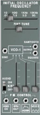
VCO 1 generates saw, square, and sine outputs. The sine output is a TimewARP 2600 extension; the original ARP 2600 VCO1 provided just sawtooth and squarewave outputs.
