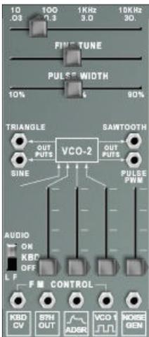
VCO 2 generates sine, triangle, sawtooth, and pulse outputs. A pulse-width slide control can adjust the duty cycle from 10% to 90%; at the middle of its travel, the pulse width is 50%, that is, a square wave.
